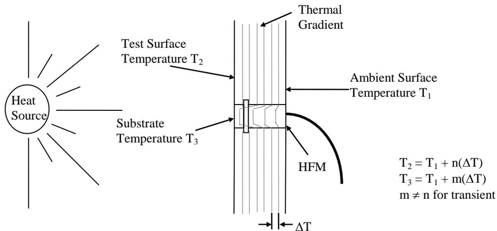
The HFM temperature sensor can be used to measure the test surface temperature once the system is in thermal equilibrium, provided that the test surface is at a uniform temperature. In such a case the temperature gradient through the HFM and the test surface will be the same because of the high thermal conductivity of the HFM.
