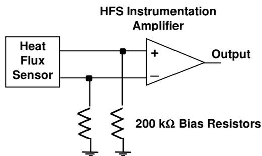
The TC channel has a switchable gain of 1, 100, 200, 500, and 1000. The circuit configuration is otherwise just like the HFS channel, i.e. with two bias resistors (200 kΩ) placed from the inputs of the amplifier to ground, etc. The TC signal may be set to zero at any desired temperature between 0°C and 250°C. See *Temperature Measurements Using the Thermocouple*.
