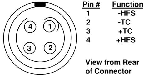
**Figure 3 - Female Lemo Connector Pin Out**
